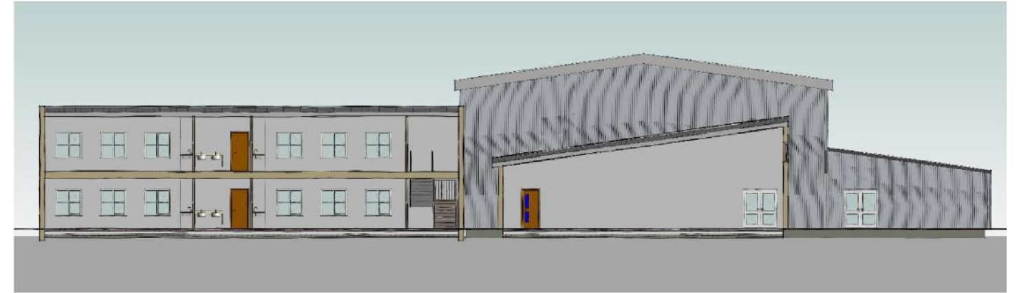
Section showing relative heights of the 2-storey teaching block, dining hall and sports hall
